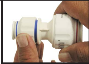
1. Twist nut counter clockwise so that color ring is exposed.
