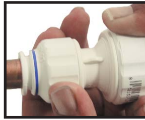
3. Twist nut clockwise until color ring disappears
